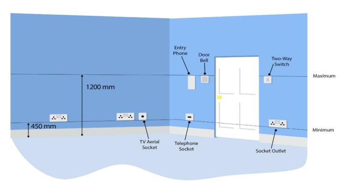
Figure C1: Height of switches, sockets etc. (See Approved Document M, section 8)
